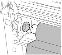
Hold the ribbon firmly while loading it, as it is easily loosened or unrolled.
